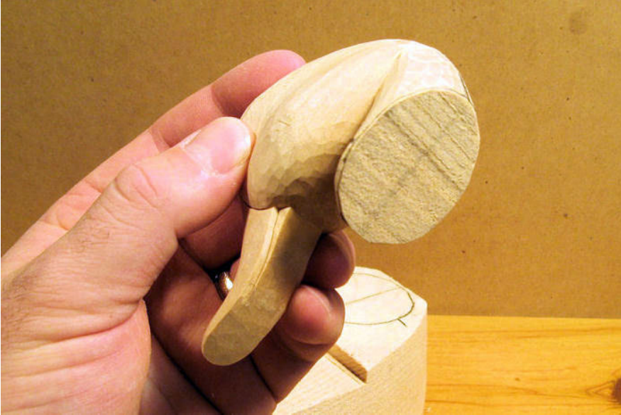
4. You can see the band saw marks remain on the base of the head at this point.
