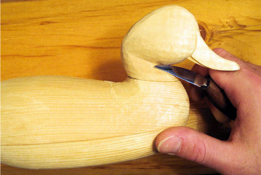
10. Use a knife to rough carve the neck into the breast, sides, and back.
